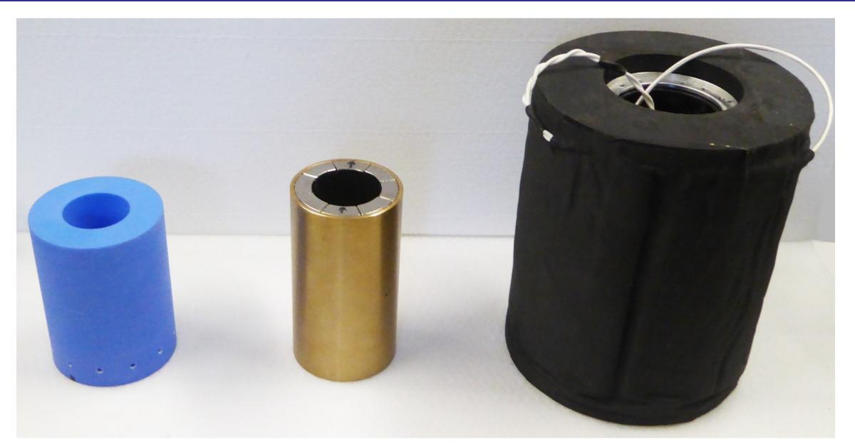
**Left:** 0.3 T 36 mm bore Mandhalas; **Middle:** 0.5 T 40 mm bore Halbach; **Right:** 0.33 T 55 mm bore shimmed Halbach;
