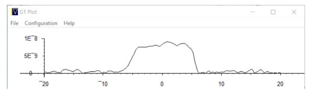
Phase-cycling has as yet not been implemented, but FFT artifacts are pleasingly low; here is the twopiece rubber sample with 0 frequency located in the glass spacer. There is no DC artifact visible at 0 frequency. A cos<sup>2</sup> window, and simple zero-padding to a power of 2 length for the FFT, are used.
