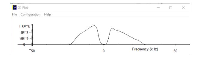
Whilst this is only 1D imaging, that is mainly due to the limitations of the magnetic gradient systems currently available to Lab-Tools; given a general 3D gradient set with drivers, full 3D imaging of modest sized objects should be possible with the Lab-Tools Mk3 NMR Spectrometer. Imaging of larger objects should be possible when the Lab-Tools Digital NMR Transmitter has completed its testing stages.
