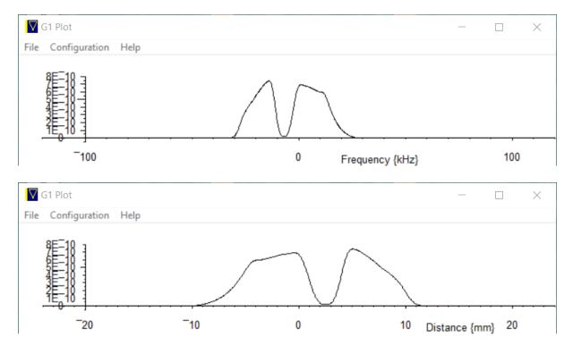
One question is why are the profiles not flat-topped ? Frequency limiting was considered, but increasing the receiver bandwidth by a factor of 10 just increased the noise, and did not change the
